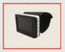
Advanced DVR which enables a second user to see and record remotely the images coming from the device, and connect to a computer with built in USB port.
